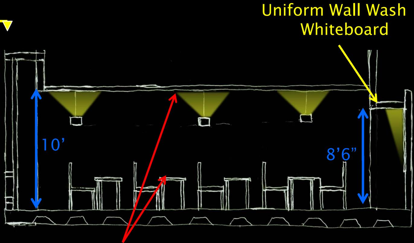
Illuminate ceiling and indirect light for task plane
